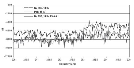
Figure 9. Dynamic range<sup>1</sup> of frequency band WR-03 (220 to 325 GHz), PNA system with and without external synthesizers<sup>2</sup> and PNA-X.
