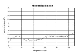
Figure 4. Plots showing residual calibration errors based on a coverage factor of 2 (2 sigma).
