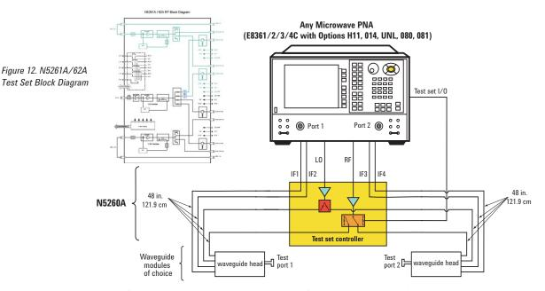
Figure 13. A banded millimeter-wave system consists of three major components: (1) Microwave PNA (E8361/2/3/4C with Options H11, 014, UNL, 080, 081) or PNA-X (N5242A with Options 200 and 020), (2) N5260A and (3) Test head modules.
