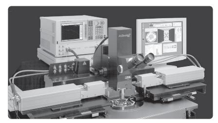
Figure 2. 110 GHz millimeter-wave system with Cascade Microtech's probe station.
