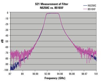
Figure 1.  $S_{21}$  filter measurement comparisons with Agilent's N5250C and 8510XF systems.
