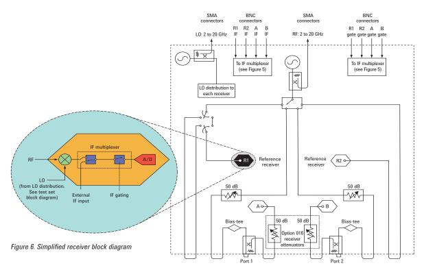
Figure 7. PNA test set block diagram
