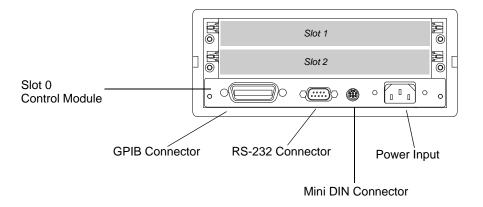
The figure below shows the Agilent 3499C rear panel. Option FP1 (1-slot) and FP2 (2-slot) filler panels can be ordered to cover any unused slots.
