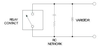
In designing RC protection networks, the protection resistor,  $R_p,$  is selected as a compromise between two values. The minimum value of  $R_p$  is determined by the maximum acceptable relay contact current (Io). The maximum allowable relay current (Io) is 2 amps ac rms or 2 amps dc. Thus, the minimum value for  $R_p$  is V/Io, where V is the peak value of the supply voltage.
