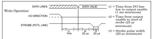
A Strobe pulse signifies that the data on the data lines is valid. During a write operation, the device receiving the data is triggered by the strobe.
