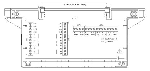
N2265A Pinout P600 is a 96-pin male DIN connector mounted on the N2265A. The connector and pinout assignments are shown below.
