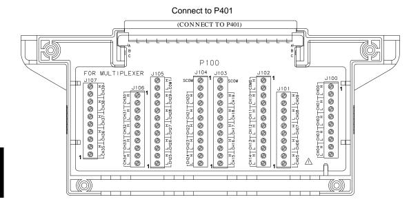
$N2260A\ Pinout\ P401$  is a 96-pin male DIN connector mounted on the N2260A. The connector and pin assignments are shown below.
