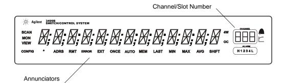
The display is divided into several areas. The channel and slot number is always displayed on the right corner of the display. The main area, which is in the center of the display, is primarily used to display channel status (open or closed), information messages, menu items, prompt information, error messages, and so on. Around the display are annunciators to indicate various states of the instrument operation. The annunciators are summarized below.
