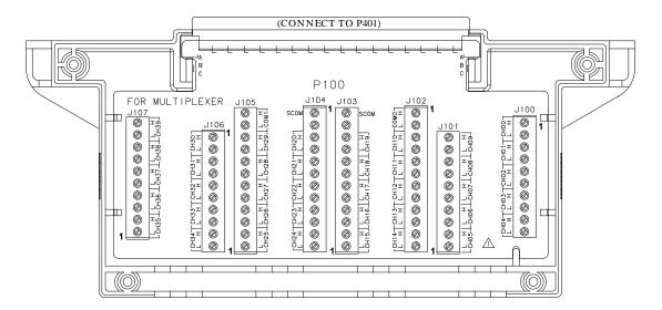
*N2266A Pinout* P401 is a 96-pin male DIN connector mounted on the N2266A. The connector and pin assignments are shown below.
