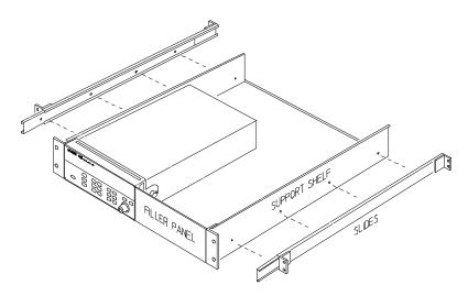
To Rack Mount a Single Agilent 3499B on a support shelf
