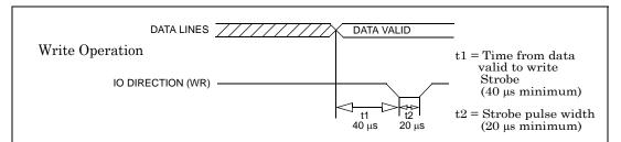
The IO Direction line is used to indicate that the data is valid on the data bus lines. IO Direction is used to trigger the receiving device.
