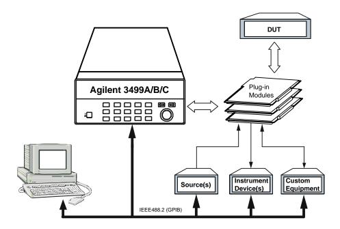
**A Typical Test System**
