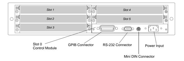
The figure below shows the Agilent 3499B rear panel.
