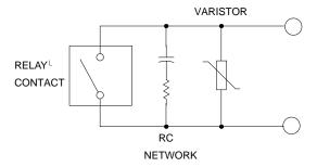
The N2267A circuit board has a provision to allow you to install protection networks in the relay paths. The figure below shows the locations on the main circuit board.
