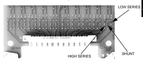
*Creating attenuators* An attenuator is composed of two resistors that act as a voltage divider. A typical attenuator circuit is also shown below.
