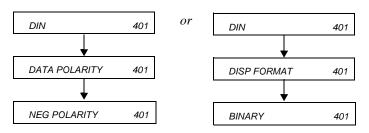
! Set the I/O Direction line polarity to negative.
