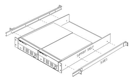
To Rack Mount Two Agilent 3499B's Side-by-side
