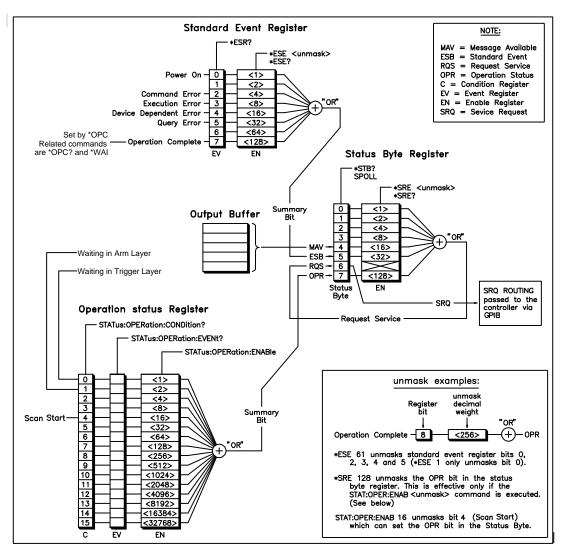
Each register group has one or more low-level registers. These low-level registers are called condition, event, or enable registers and control the action of specific bits in the registers. You read or write to the registers using binary-weighted decimal numbers.
