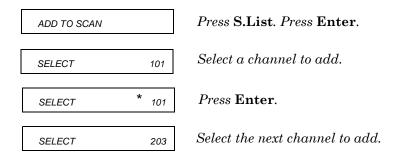
Remote Interface Operation: You may use single channels, ranges of channel, or stored setups in the scan list. Set up a scan list with one command as follows:
