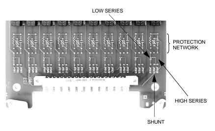
*Protection Networks* An RC protection network and a varistor can be installed in each relay path. More detailed information about protection circuits is given on page 272.
