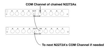
You can also connect multiple N2272A's in a tree structure to implement high channel count multiplexers, however, this configuration will cause signal delays.
