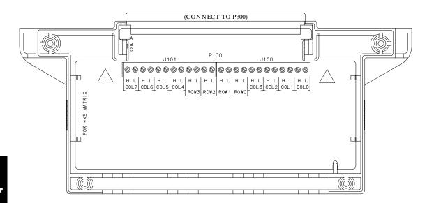
N2262A Pinout P300 is a 96-pin male DIN connector mounted on the N2262A. The connector and pinout assignments are shown below. Note that the A and B rows in the connector are not used.
