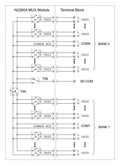
1-Wire Mode In this mode, either the High (H) or Lo (L) terminal of a channel is switched to the single-ended (SE-COM) terminal. The Lo terminals form the first 40 1-wire channels (00-39), and the Hi terminals form the second 40 1-wire channels (40-79). Only one channel can be closed at a time in the 1-wire mode.
