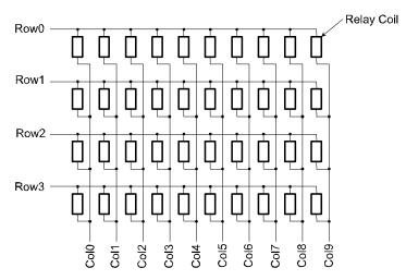
The 3499A/B/C/C/C supports parallel operation of latching relays. Any relay in the same row can be opened or closed at the same time. Basically, the relays are switched row by row, or bank by bank.
