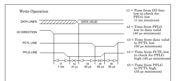
The complete handshaking sequence for Mode #5 is as follows: The 3499A/B/C checks to see if the receiving device has set the PFLG line low, this indicates the receiving device is ready to accept data. When PFLG is low, the 3499A/B/C sets the data on the data bus and sets PCTL low. The 3499A/B/C then waits for the receiving device to set PFLG high, indicating that it has latched the data. To complete the handshake, the 3499A/B/C sets PCTL high.
