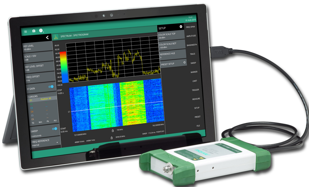
Figure 2-11. MS276xA Connection to Tablet
