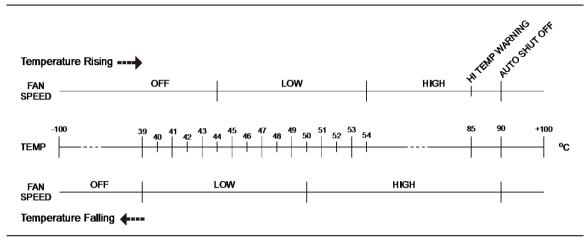
Figure C-1. Fan Speed versus Temperature
