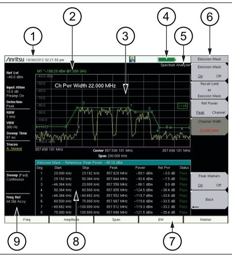
Figure 2-8. Spectrum Analyzer Display
