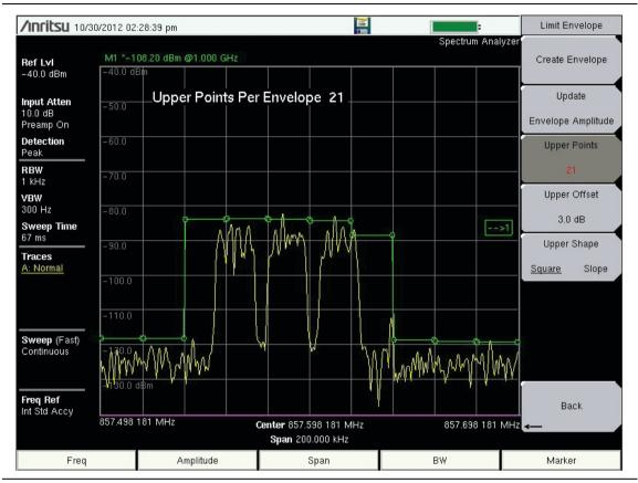
Figure 3-1. Complex Limit Line Example
