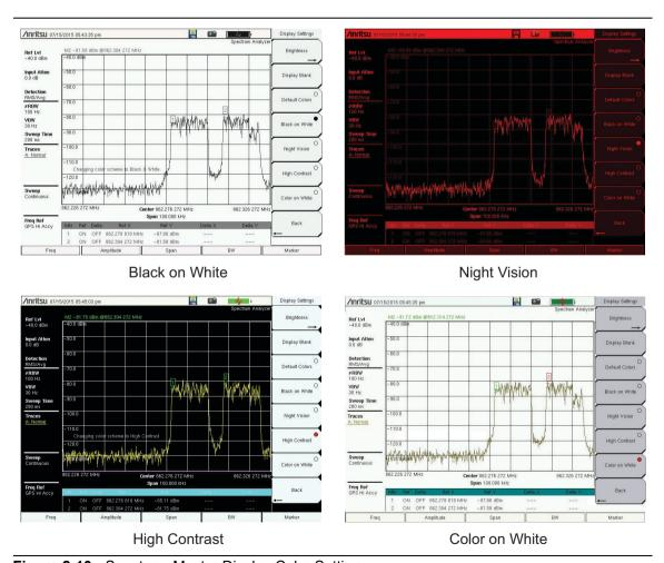
Figure 2-10. Spectrum Master Display Color Settings
