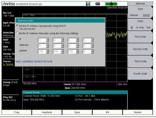
Figure D-3. IP Address Assigned Using DHCP
