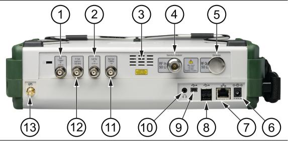
Figure 2-6. Test Panel Connectors for MS2720TOptions 709, 713, 720
