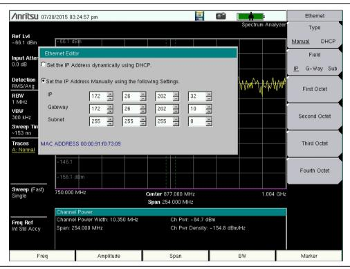
Figure D-2. Setting IP Address Manually
