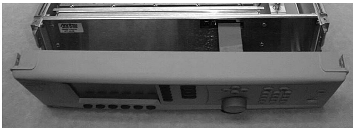
Figure 7-4. Front Panel Removal
