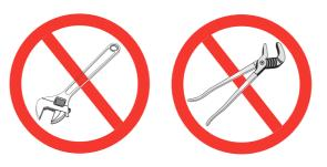
Figure E-8. Do Not Use Pliers or Adjustable Wrenches
