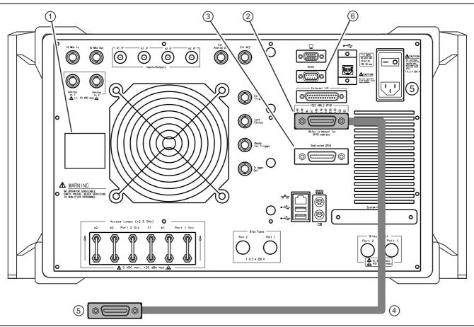
Figure 4-2. VNA Rear Panel GPIB Cable connection to the IEEE 488.2 GPIB Port
