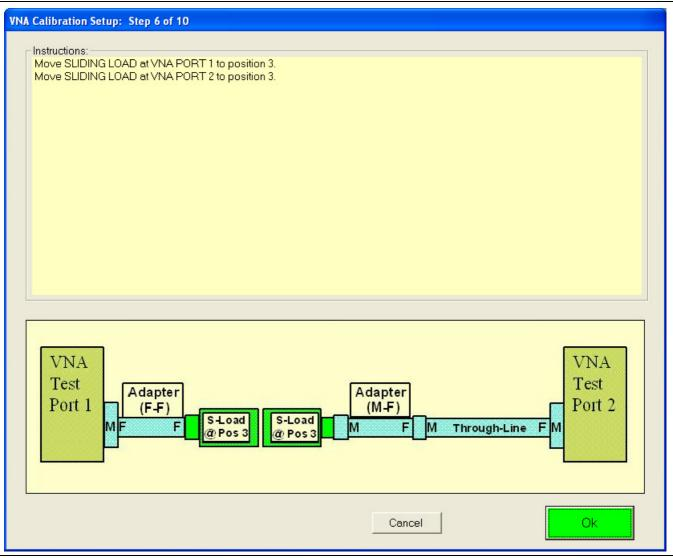
Figure 6-24. VNA Calibration Setup – Sliding Loads – Step 6 of 10
