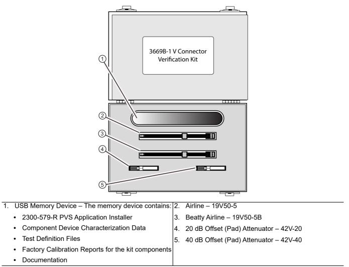
Figure 1-1. 3669B-1 V Connector Verification Kit Contents
