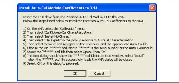
Figure 6-34. Install AutoCal Module Coefficients Dialog Box
