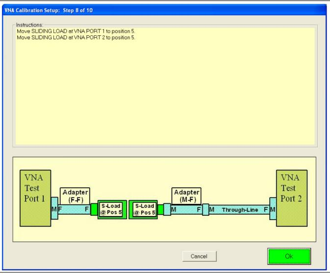
Figure 6-26. VNA Calibration Setup – Sliding Loads – Step 8 of 10
