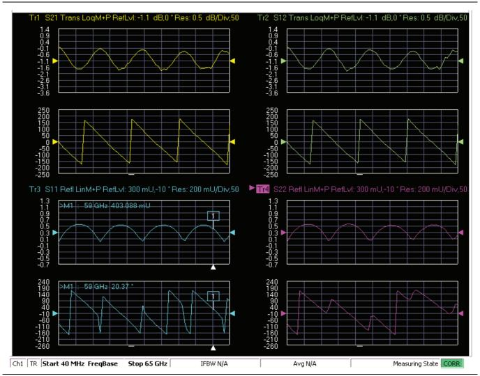
Figure 6-46. MS4640A/B Series VNA, Typical Mismatched Thru Data in Low Band
