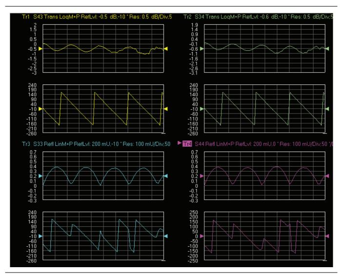
**Figure 5-80.** MS4640B Series VNA, Typical Mismatched Thru Data in Low Band Upper-left quadrant= S43 – Forward Transmission Upper-right quadrant= S34 – Reverse Transmission Lower-left quadrant= S33 – Forward Reflection Lower-right quadrant= S44 – Reverse Reflection
