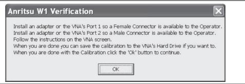
Figure 7-10. Anritsu W1 Verification – Install Adapter (F out) on Port 1 – Install Adapter (M out) on Port 2
