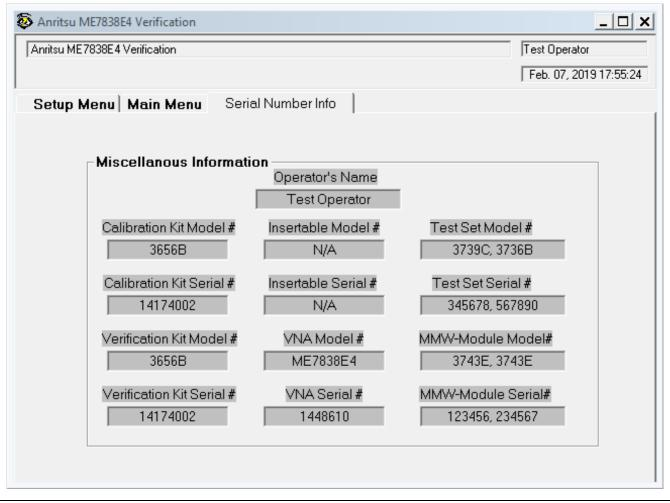
Figure 5-72. ME7838E4 Application Interface – Serial Number Tab
