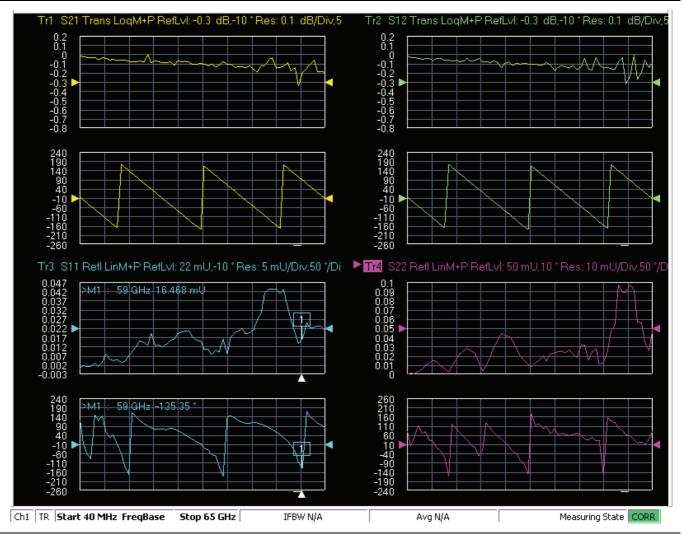
**Figure 3-42.** MS4640B Series VNA, Typical Matched Thru Data in Low Band Upper-left quadrant= S21 – Forward Transmission Upper-right quadrant= S12 – Reverse Transmission Lower-left quadrant= S11 – Forward Reflection Lower-right quadrant= S22 – Reverse Reflection
