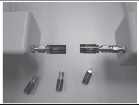
Figure 7-12. Calibration Device Connections
