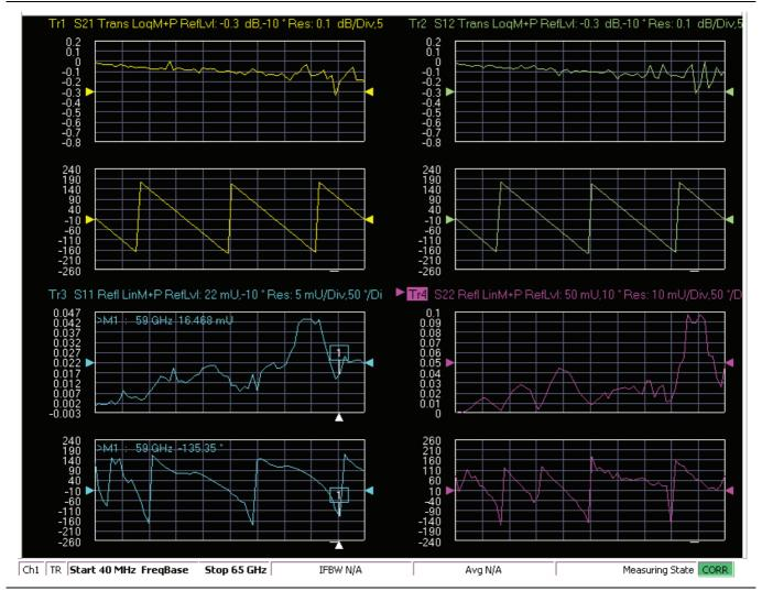
**Figure 6-42.** MS4640A/B Series VNA, Typical Matched Thru Data in Low Band Upper-left quadrant= S21 – Forward Transmission Upper-right quadrant = S12 – Reverse transmission Lower-left quadrant= S11 – Forward Reflection Lower-right quadrant= S22 – Reverse Reflection
