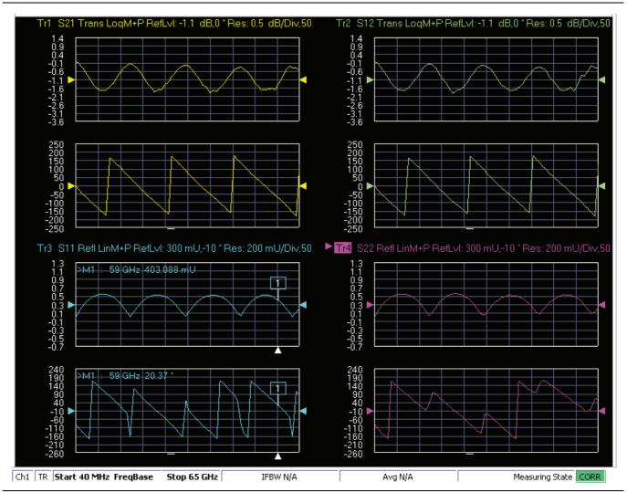
Figure 5-53. MS4640B Series VNA, Typical Mismatched Thru Data in Low Band
