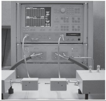
Figure 7-1. VNA Calibration and Measurement Setup
