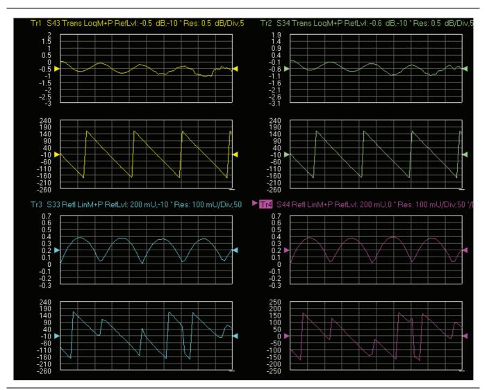
**Figure 4-80.** MS4640B Series VNA, Typical Mismatched Thru Data in Low Band Upper-left quadrant= S43 – Forward Transmission Upper-right quadrant= S34 – Reverse Transmission Lower-left quadrant= S33 – Forward Reflection Lower-right quadrant= S44 – Reverse Reflection
