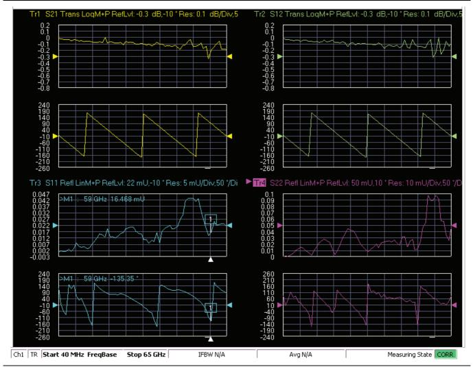
**Figure 2-43.** MS4640A/B Series VNA, Typical Matched Thru Data in Low Band Upper-left quadrant= S21 – Forward Transmission Upper-right quadrant= S12 – Reverse Transmission Lower-left quadrant= S11 – Forward Reflection Lower-right quadrant= S22 – Reverse Reflection
