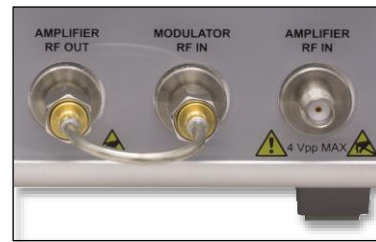
Figure 7 Amplifier RF Out present only on the MX10B series of transmitters. This cable is not installed on the MX40B transmitter series.
