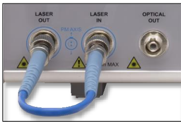
Figure 6 PM Loopback Fiber Cable Installed
