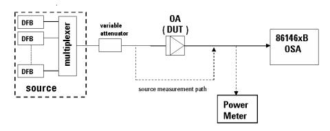
Figure 1 Patch cord used to bypass the DUT
