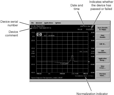
Normalization indicator The time interval between normalizations can be set from the specification file
