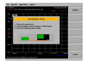
4 Follow the on-screen instructions to perform the source normalization. After the source normalization is successfully completed, press Continue to return to the previous menu. The device under test can be measured. See "To measure the device under test" on page 3-14.
