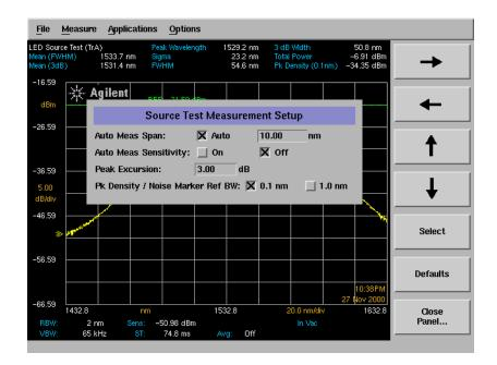
Auto Measure (Auto Meas) Span selects the wavelength span for viewing the signal located by the auto measure function. If Auto is specified, the span is set wide enough to display most of the signal. If a particular span is desired, clear
