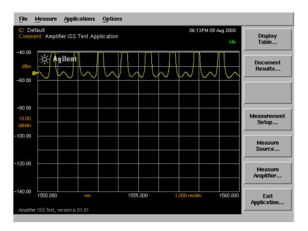
c A third sweep measures the noise level, indicated by "Source Noise Sweep...".
