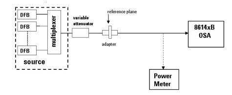
To calculate offsets in a standard measurement setup
