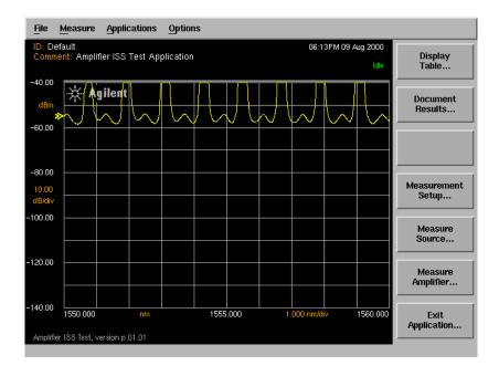
5 When the measurement is complete, the MEASURE AMPLIFIER... softkey is enabled. The progress status label reads "Idle".
