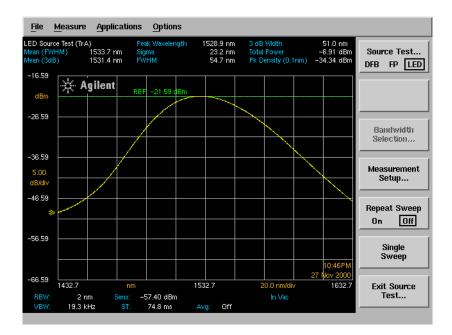
6 Press Auto MEAs to locate and display the laser's response automatically.
