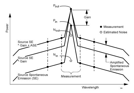
The noise figure of the amplifier is calculated from the measurements of the signal and ASE power levels using the following equations:
