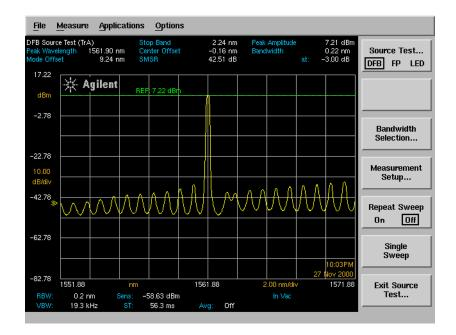
The Source Test results panel appears in the marker area at the top of the screen. Measurement results (attributes) for all source tests are displayed in this panel. The currently selected source test and trace names are displayed in the upper left corner of the results panel. Once a source test is initiated on a given trace, it remains associated with that trace even though another trace may be made active.
