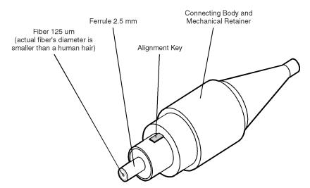
Figure 1 Basic components of a connector.
