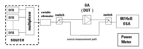
Figure 2 Optical Switches to bypass the DUT
