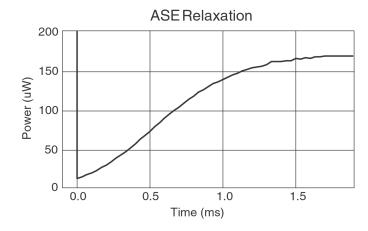
Figure 8 ASE time domain characteristics
