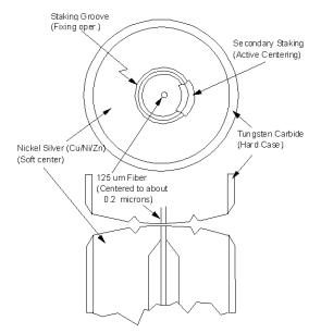
The HMS-10 encases the fiber within a soft nickel silver (Cu/Ni/Zn) center which is surrounded by a tough tungsten carbide casing, as shown in Figure 3.
