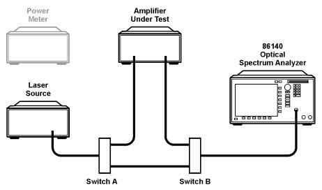
Figure 6 Amplifier Measurement
