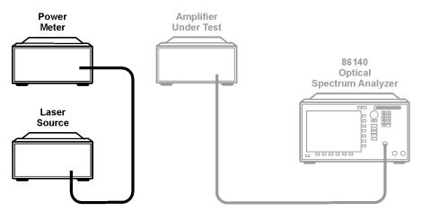
Figure 4 Power Meter Measurement
