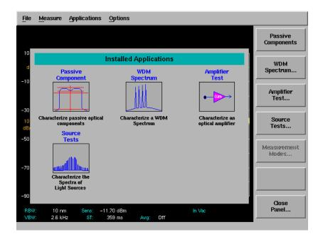
Each installed application has an icon on the panel and a corresponding softkey.
