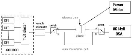
Figure 5 Source Path Measurement
