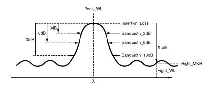
Example 5-4 on page 3-49 shows a specification set written to characterize a WDM filter. The specification set measures the insertion loss, the 3 dB, 6 dB, and 10 dB bandwidths, the peak wavelength and the crosstalk.
